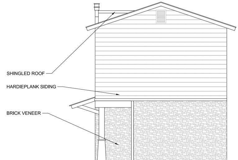
3B - 1H - 2G SIDE ELEVATION - SCALE: 1/4" = 1'-0"
