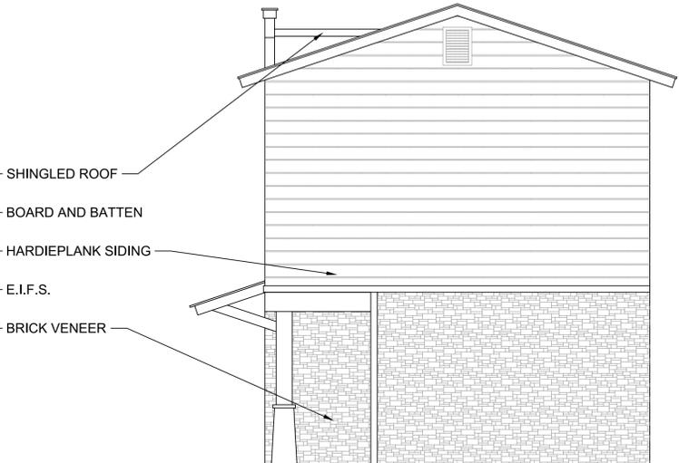
————— SCALE: 1/4" = 1'-0" SIDE ELEVATION ————— SCALE: 1/4" = 1'-0"
