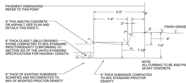
2'-0" CONCRETE CURB & GUTTER NOT TO SCALE
