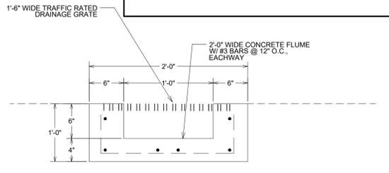
**CONCRETE TRENCH DETAIL** NOT TO SCALE
