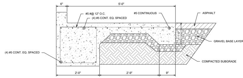
CONCRETE VACCUM FOOTING DETAIL NOT TO SCALE
