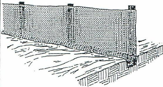
4. Backfill and compact the excavated soil.
