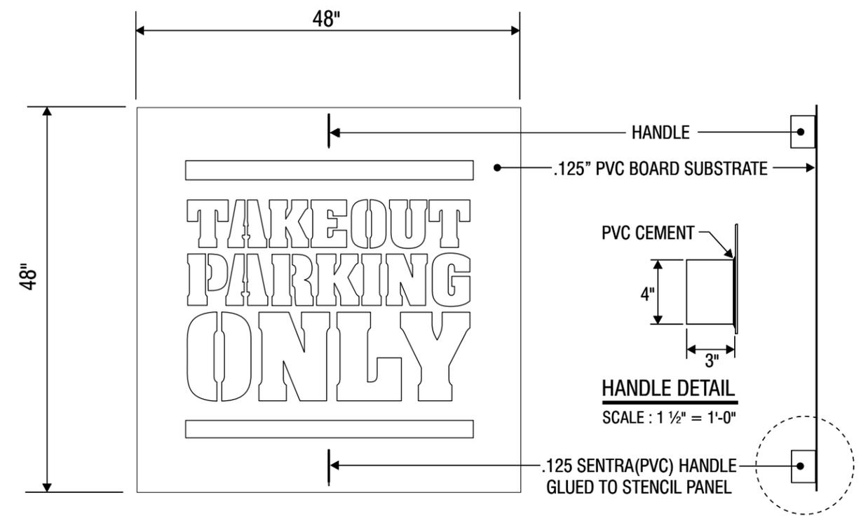
**MANUFACTURE ONE (1) PARKING LOT STENCIL AS SHOWN AND NOTED. STENCIL FABRICATED OUT OF .125 PVC BOARD (SENTRA OR EQUIV). GRAPHICS ROUTED-OUT OF PVC BOARD. HANDLES GLUED ONTO STENCIL BOARD FOR STENCIL REMOVAL.**
