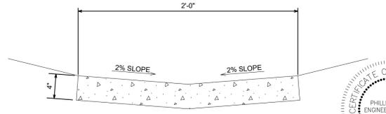
**CONCRETE TRICKLE CHANNEL** NOT TO SCALE
