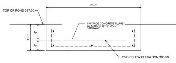
**OVERFLOW STRUCTURE DETAIL** NOT TO SCALE
