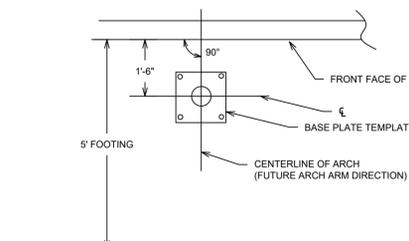
BASEPLATE TEMPLATE ORIENTATION DETAIL NOT TO SCALE
