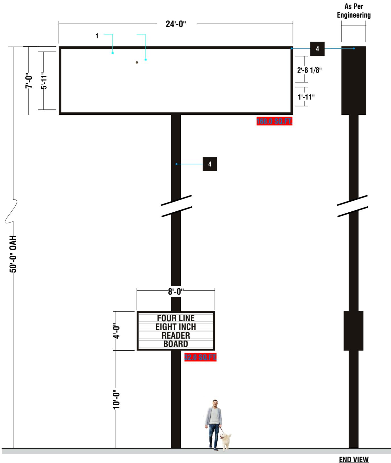
**A CUSTOM D/F INTERNALLY ILLUMINATED PYLON SIGN W/ READER BOARD | 200.0 SQ.FT.**
