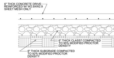
CONCRETE DRIVE SECTION NOT TO SCALE
