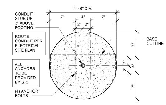
DTE EXIT SIGNAGE BOLT PATTERN (TOP VIEW)
