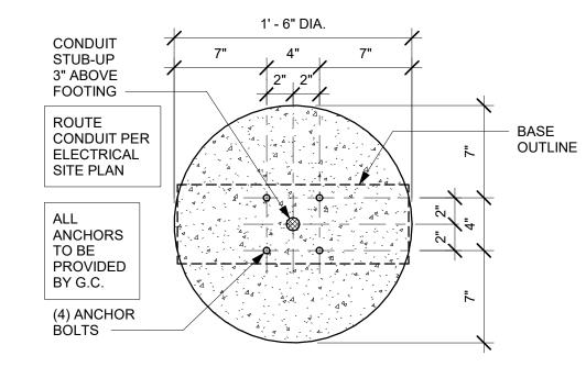
5 DTE ARROW SIGNAGE BOLT PATTERN (TOP VIEW)
