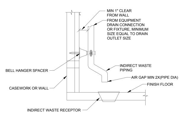
WALL SPACER HANGER SPECIFICATION: COPPER PLATED OR CORROSION RESISTANT BELL HANGER, WARWICK SERIES 300, OR EQUIVALENT PRODUCT.
