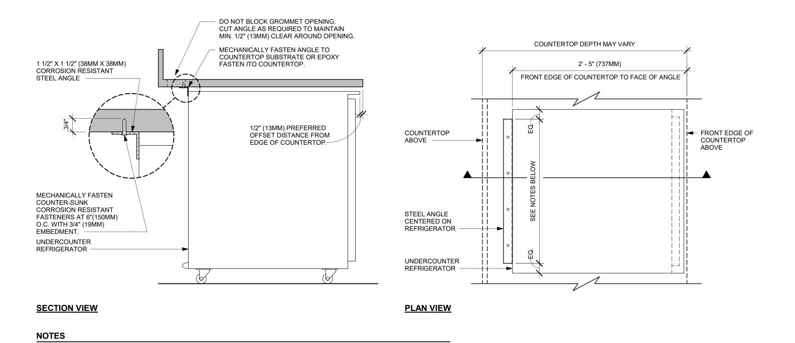
1. 24" (610MM) 1 1/2" X 1 1/2" (38MM X 38MM) STEEL ANGLE TO BE USED WITH SINGLE DOOR REFRIGERATORS.
