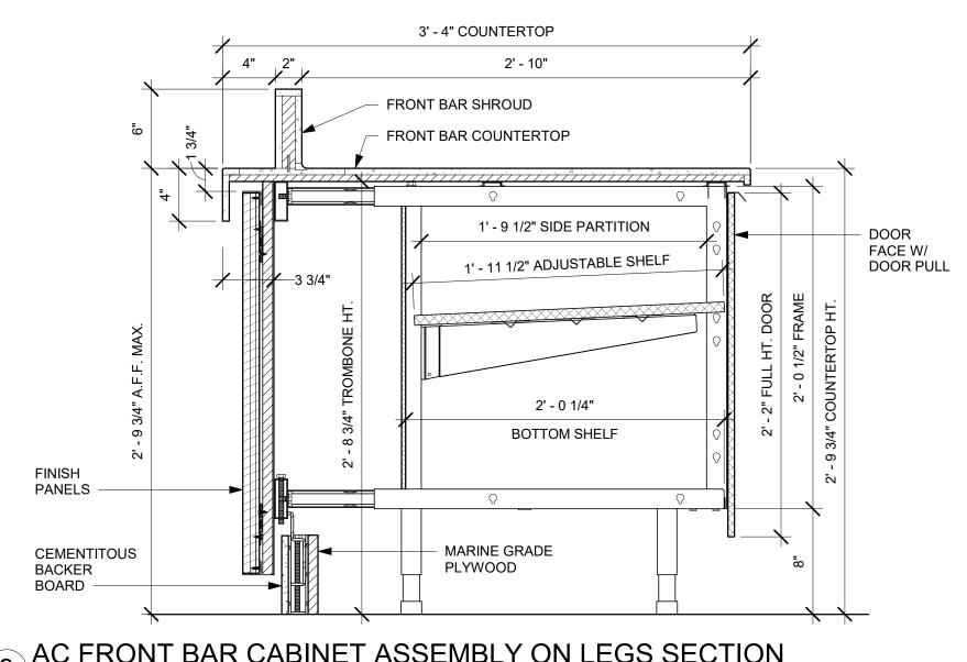
3 AC FRONT BAR CABINET ASSEMBLY ON LEGS SECTION
