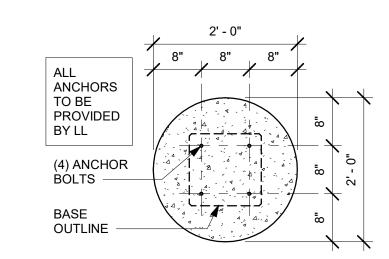
9 DTE CLEARANCE BAR BOLT PATTERN (TOP VIEW)
