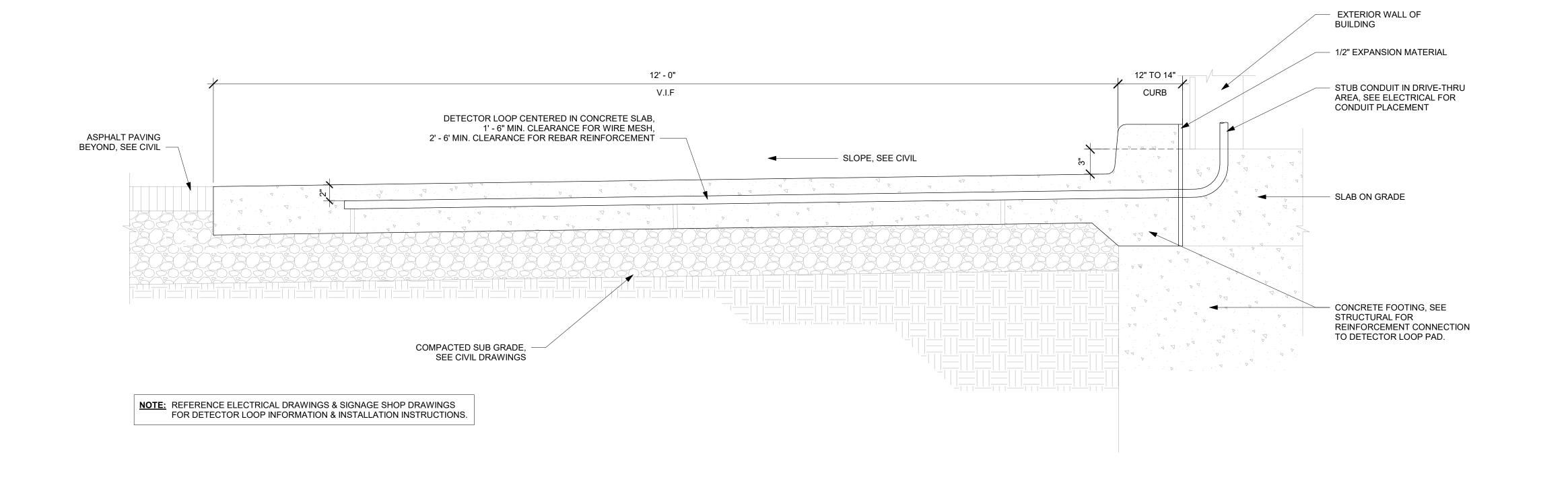
SECTION @ DETECTOR LOOP IN CONCRETE PAD AT DRIVE-THRU WINDOW
