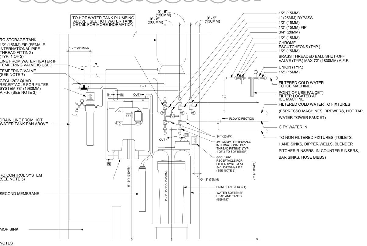
6. COMPONENTS ARE TO BE POSITIONED TO MAXIMIZE ACCESS FOR REGULAR SERVICING. PRE-FILTER, BYPASS VALVES, AND SOFTENER TANKS MUST BE INSTALLED 72" (1828MM) AFF OR LOWER.
