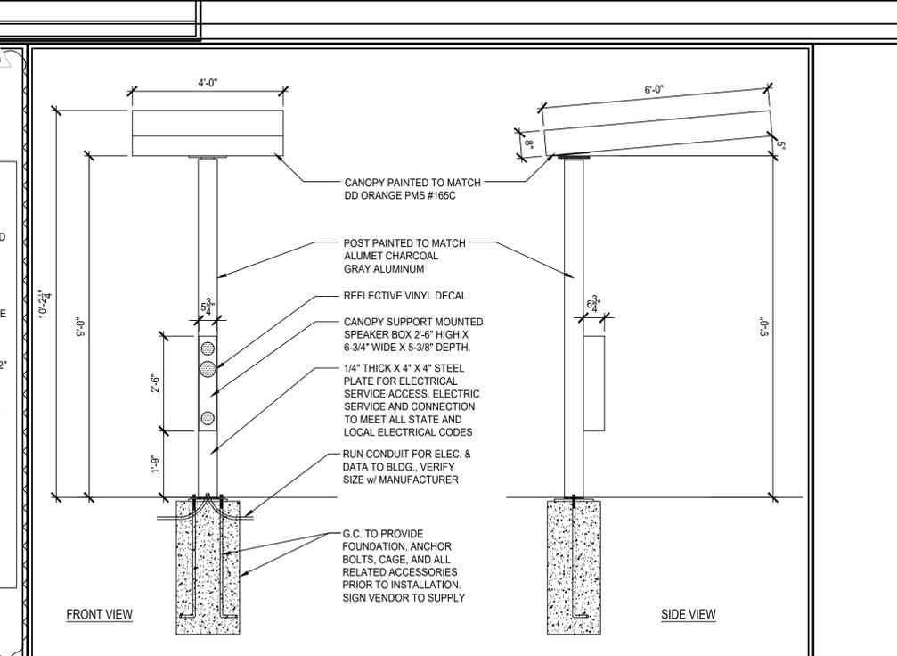
**1 DUAL & SINGLE VEHICLE CLEARANCE BAR DETAIL**
