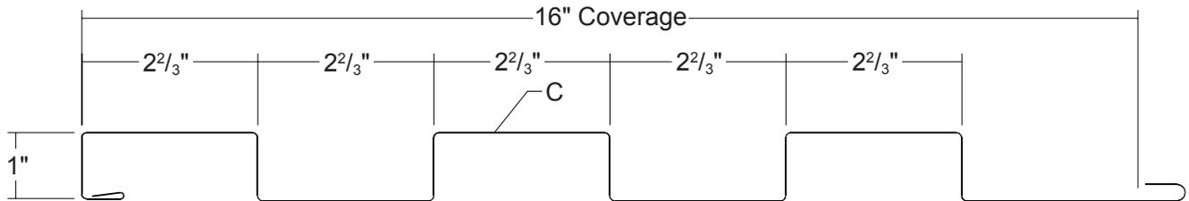
Panel can be produced in lengths from 5' to 30'.
