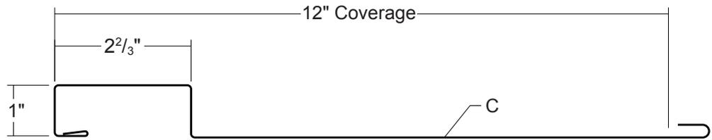
Panel can be produced in lengths from 5' to 30'.
