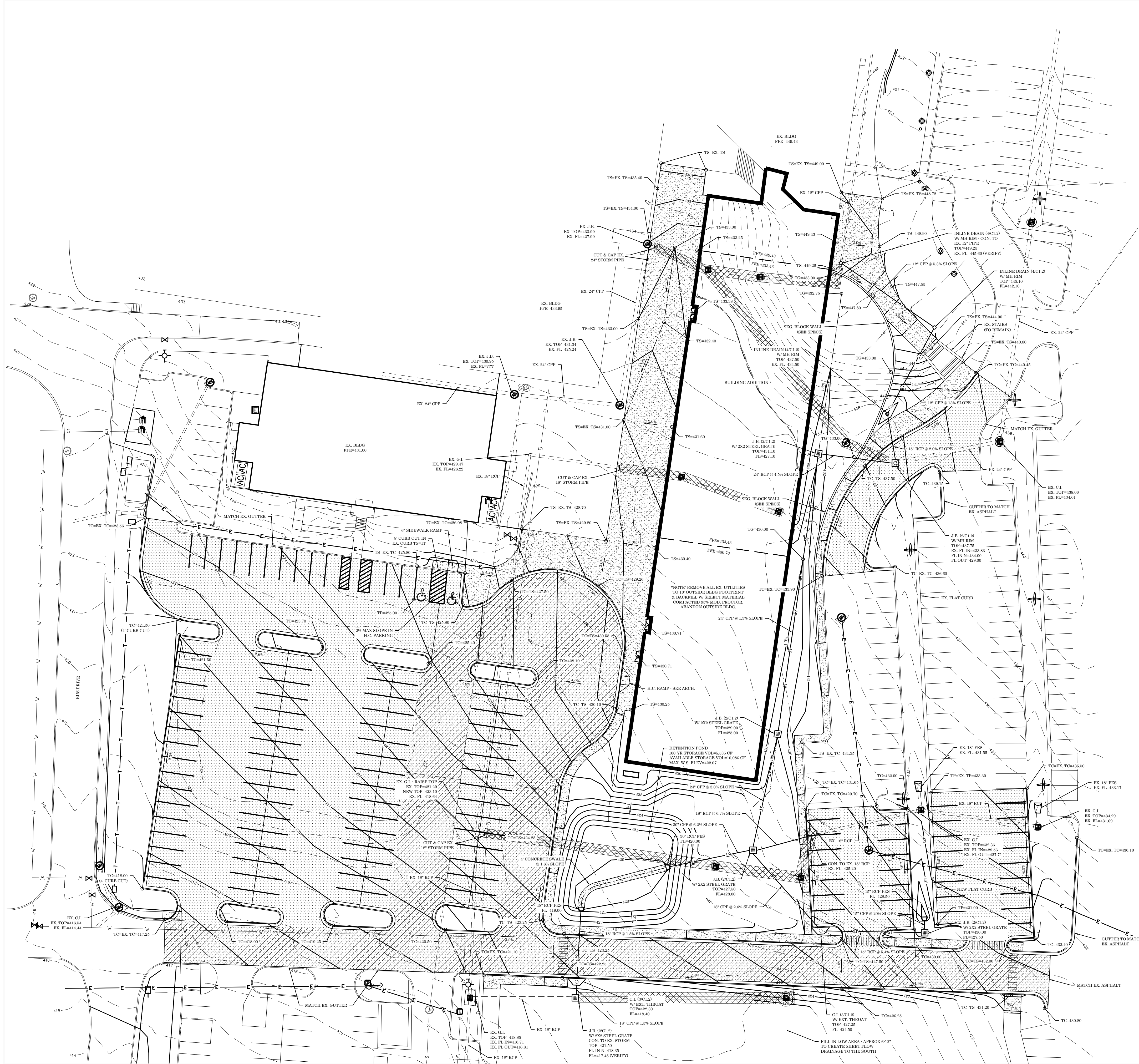
1 SITE GRADING & STORM DRAINAGE PLAN SCALE: 1" = 30' 0 30 60
