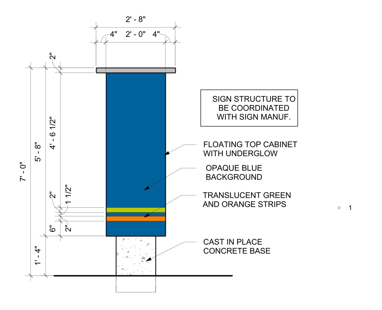
ELECTRICAL FOR INTERNALLY LIT CABINET TO BE PROVIDED BY GC. LIGHTING TO BE PROVIDED AND INSTALLED BY SIGN MANUFACTURER
