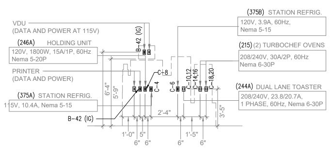
7'-10" SANDWICH STATION ELEVATION E-2 | SCALE: 1/4"=1'-0"
