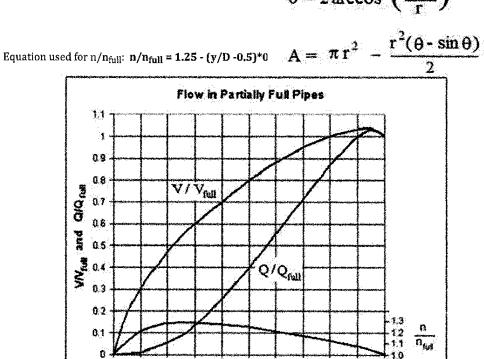
Flow In Partially Full Pipes
