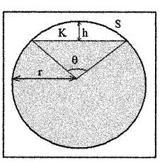
Partially Full Pipe Flow Parameters (More Than Half Full) Р
