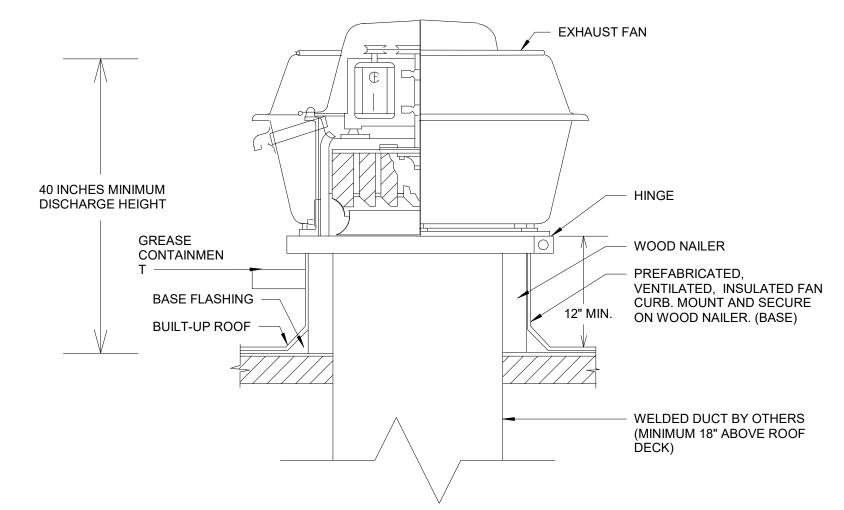
4 ROOF MOUNTED GREASE EXHAUST FAN SCALE: N.T.S.
