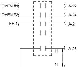
NOTE: HOOD CONTROLS SHALL OPERATE SUCH THAT AUTOMATIC HEAT SENSOR OR THE MANUAL EVACUATION BUTTON WILL ENERGIZE THE EXHAUST FAN AND DE-ENERGIZE THE EQUIPMENT UNDER THE HOOD AS WELL AS THE GAS SERVING THE PIZZA OVEN. CONTRACTOR SHALL PROVIDE ALL LABOR AND MATERIALS AS REQUIRED FOR A COMPLETE FUNCTIONAL SYSTYEM.
