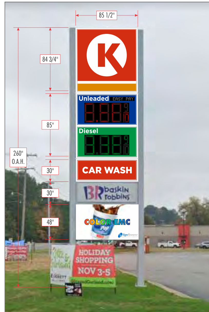
PROPOSED LEDS SIZES: NEW 24" RED/GREEN ABLE 7-SEG. LEDS SIZES SUBJECT TO FINAL FIELD CONFIRMATION PRIOR TO MANUFACTURING
