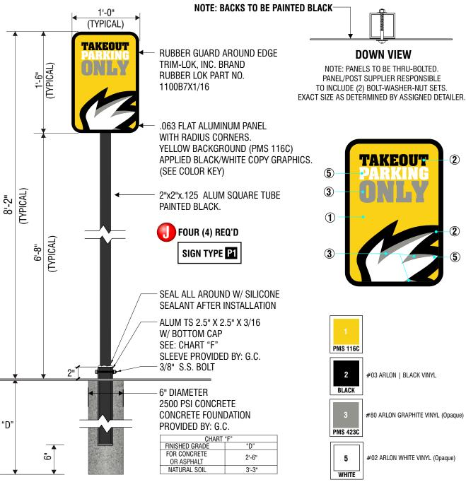
**NOTE: TO BE USED ONLY WHEN** THE SIGN IS PLACED ON A SIDEWALK OR SIMILAR CONCRETE SURFACE.
