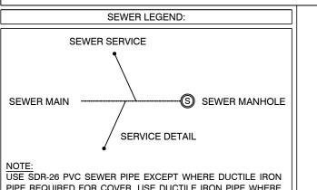
USE SDR-26 PVC SEWER PIPE EXCEPT WHERE DUCTILE IRON PIPE REQUIRED FOR COVER. USE DUCTILE IRON PIPE WHERE 3' MINIMUM COVE CANNOT BE MAINTAINED. CONTRACTOR IS RESPONSIBLE FOR LOCATING ALL BURIED UTILITIES PRIOR TO CONSTRUCTION.
