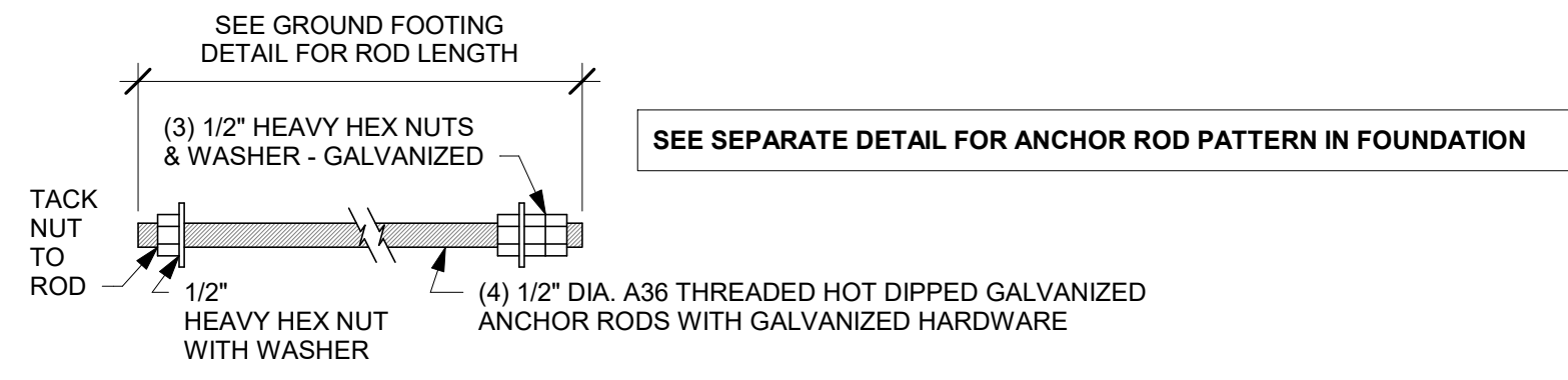
7 DTE 5-PANEL MENU BOARD ANCHOR ROD Scale: 3" = 1'-0"
