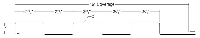
Panel can be produced in lengths from 5' to 30'.
